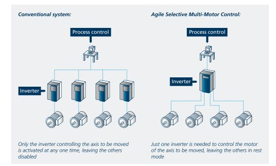
By using two digital inputs in binary combination mode, users can activate the inverter's parameter configuration corresponding to just one of the four motors, thus excluding the other three.
