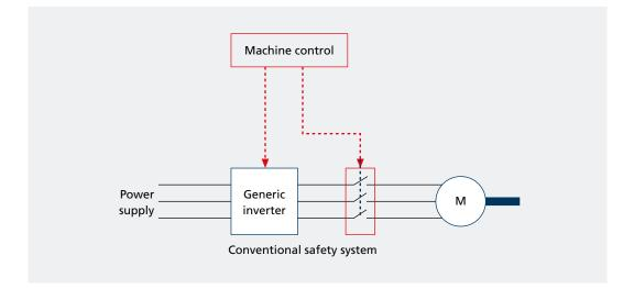
Bonfiglioli has integrated the Safe-Torque-Off system (STO, EN61800-5-2) in Agile inverters to reduce the size of control panels, minimise the number of operating components, simplify control, and eliminate the mechanical stress caused by the sudden application of the brake while the shaft is still turning. In an emergency this system disconnects the motor in compliance with EN13849-1 PL d and EN61508 SIL2, without the need for external contactor.
